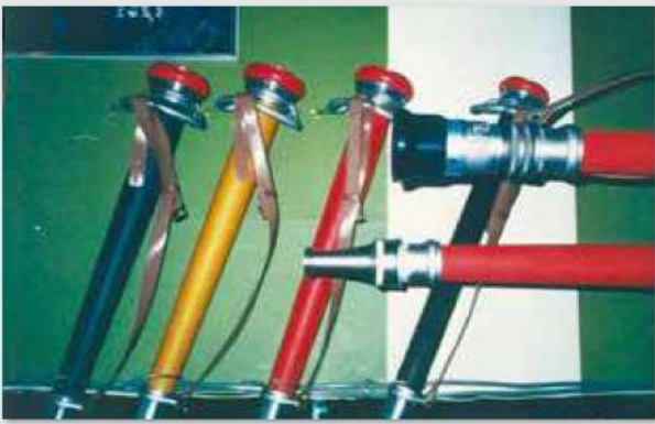
Firefighting hose (grooved) (NPE)
