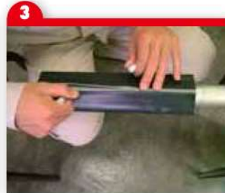
3 Apply the tube and mate the fastener parts while applying instant adhesive.
